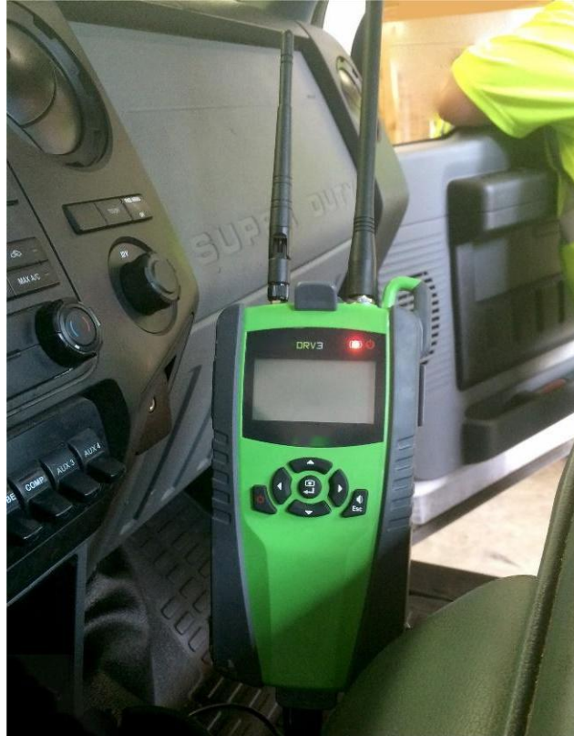
Figure 8: Docking station used in service vehicle
